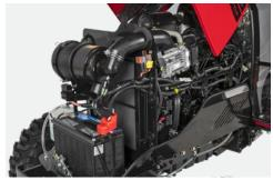
**EASY MAINTENANCE**Lift-up hood and side panels allows for easy access to battery, air filter, and fuel tank. Servicing your tractor is as easy pushing a button.
